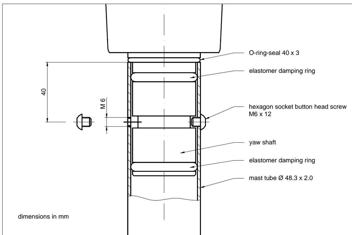
With this configuration the attached plastic bushing is not needed. For easy assembling the two damping rings of the yaw shaft and the inside of the mast tube should be lubricated with Vaseline or grease. Now insert the yaw shaft into the tube and push it until the O-ring seal 40x3 seats solidly at the face side of the tube. Please take care not to damage the damping rings during feeding in.
