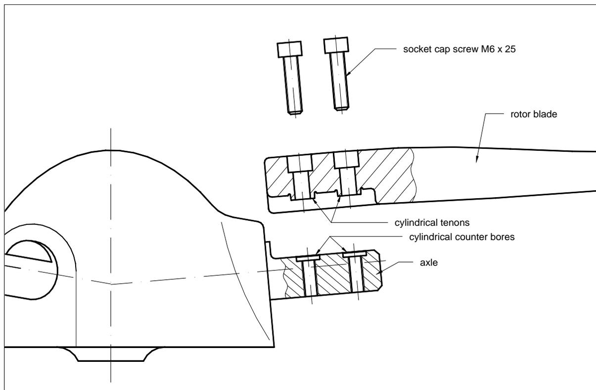
The rotor blades are fixed by two socket cap screws M6 x 25, which are TUFLOK-coated to prevent loosening at operation. When screwing in you will sense a slight drag torque due to the coating.
