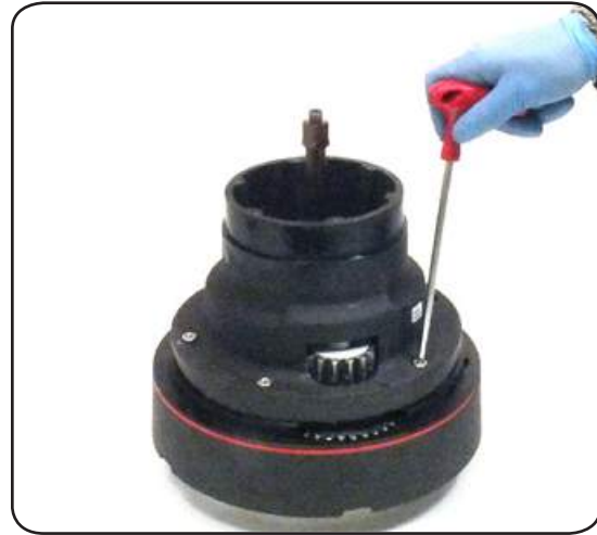
12. Unscrew the six screws n°22
