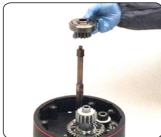
15. Slide out the assy ratchet hub 2nd speed
