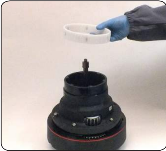
11. Slide out the roller bearings n°18
