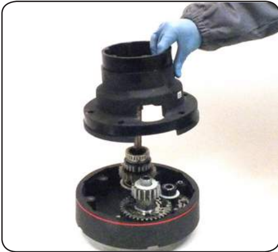
13. Slide out the drum support n°15
