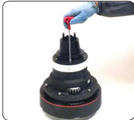
8. Unscrew the six screws n°23
