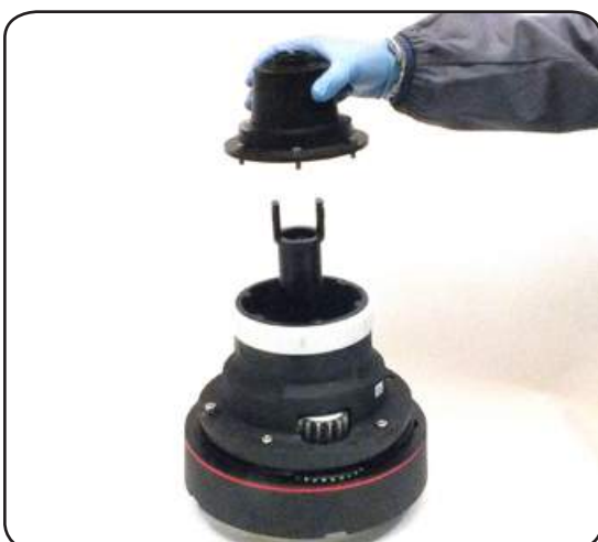
9. Slide out the assy flange n°19
