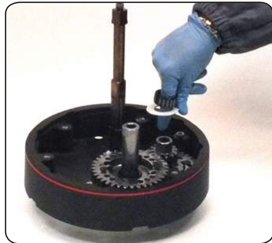
19. Remove the roller bearing n°2 and the washer n°10
