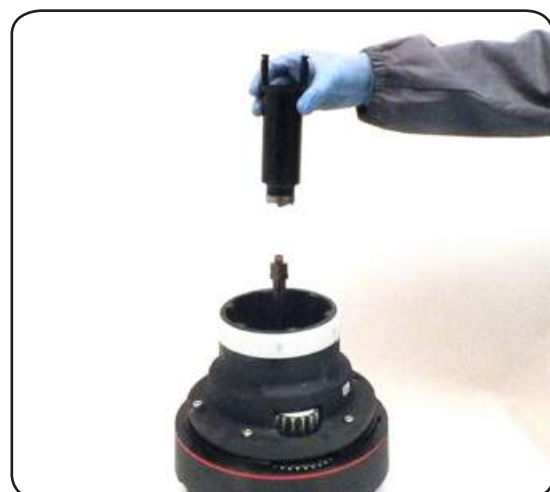
10. Slide out the assy command tube n°31
