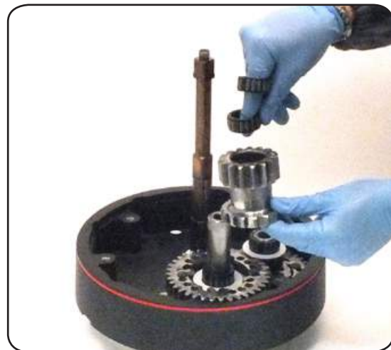
17. Slide out roller bearings n°2 and gear n°13
