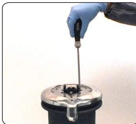
4. Unscrew the three screws n°43
