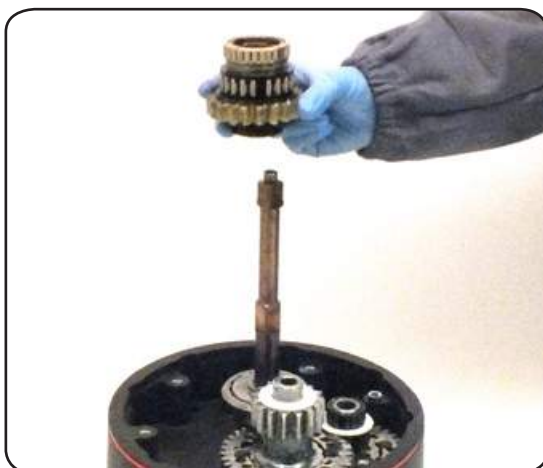
14. Slide out the assy clutch 3rd speed
