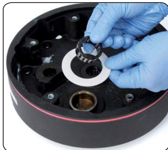
22. Remove the roller bearing n°6 and the washer n°11
