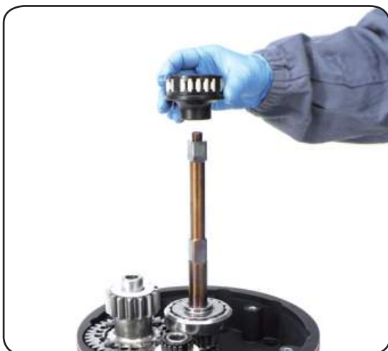
9. Slide out the inner spacer n°34 and the roller bearing n°23
