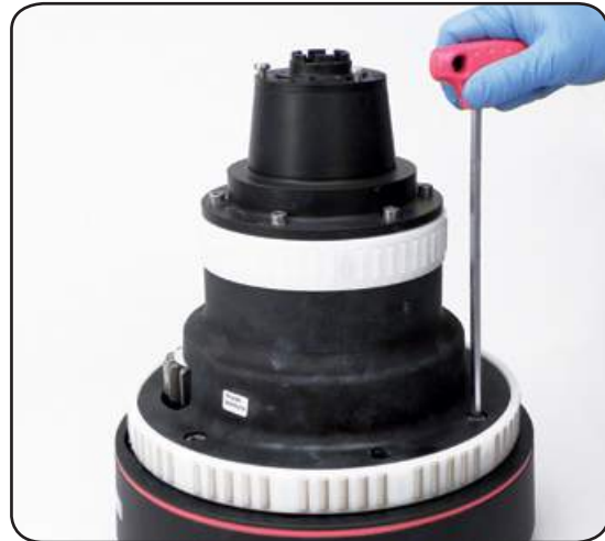
6. Completely unscrew the six screws n°25 ( \approx 20\text{Nm}/177\text{ in-lb} )
