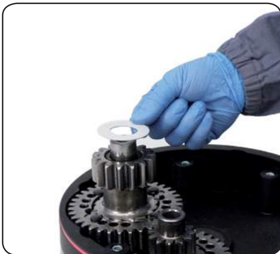
15. Slide out the washer n°5
