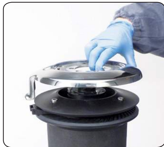
4. Unscrew the three screws n°37 (⚙️ 4Nm/35 in-lb) and remove the stripper arm n°36 by rotating and lifting it.
