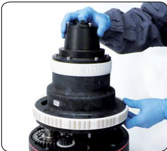
7. Lift off the assy housing n°18
