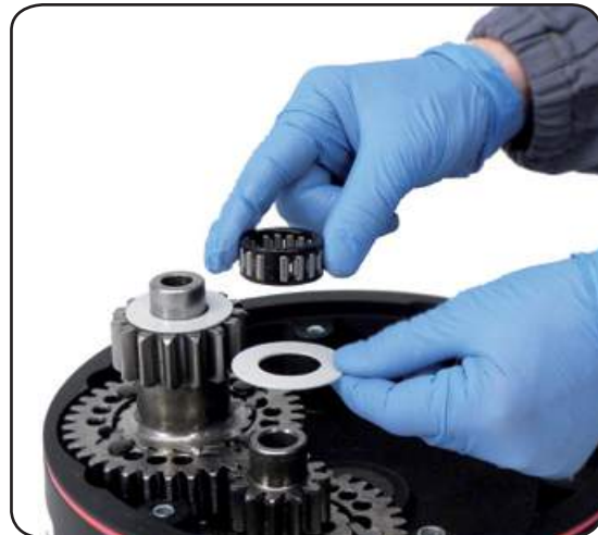
14. Slide out the roller bearing n°6 and the washer n°5
