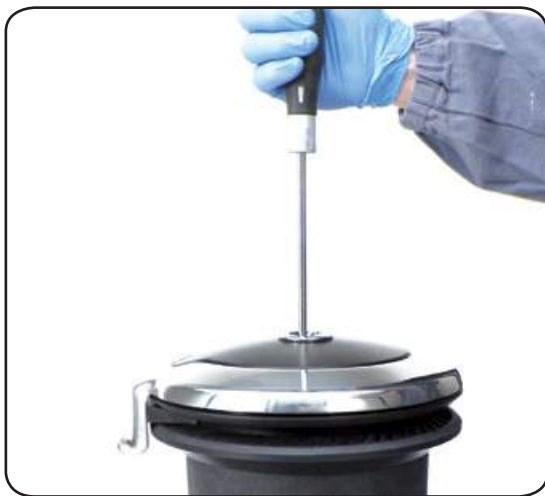
1. Unscrew the central screw (⚙️ 2Nm/18 in-lb)
