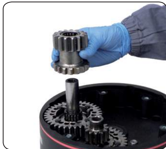
16. Slide out the final drive pinion n°9
