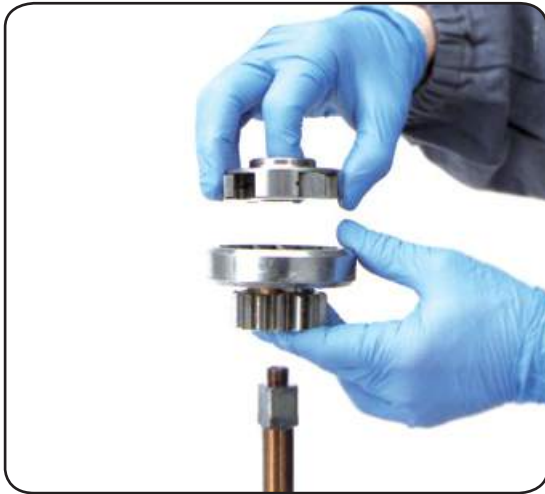
11. Disassemble the Assy pinion n°33 and the hub n°32
