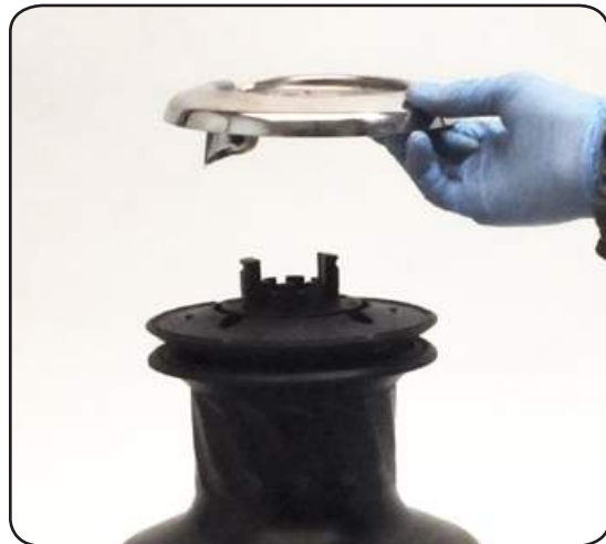
4. Remove the self-tailing arm n°27 by rotating and lifting it.
