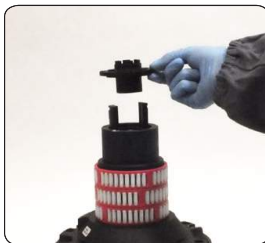
6. Remove the stripper arm housing n°21
