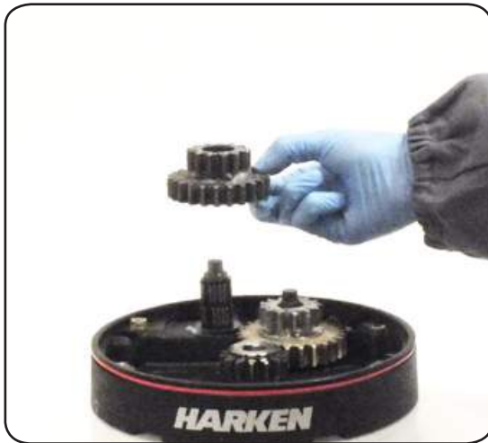
13. Remove the idler and pinion n°14
