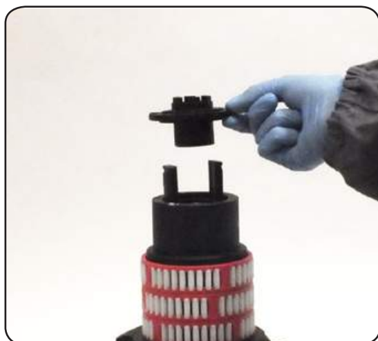
6. Remove the stripper arm housing n°21
