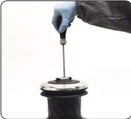
1. Unscrew the central screw (🔧2Nm/18 in-lb)
