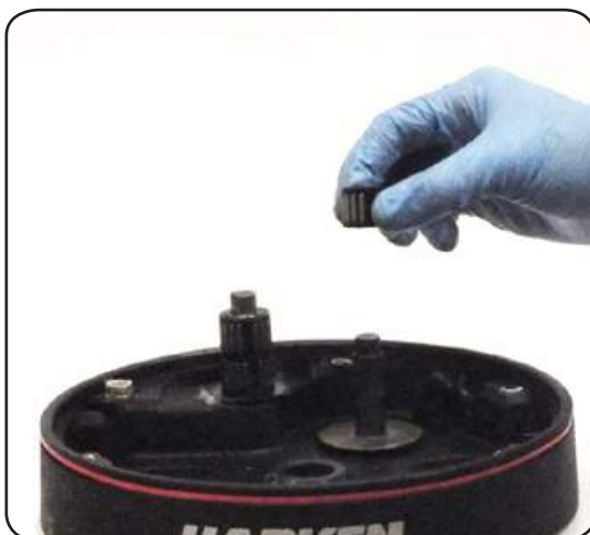
17. Remove the roller bearing n°12
