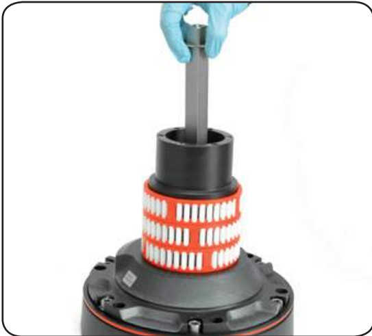
8. Slide out the central shaft n°19
