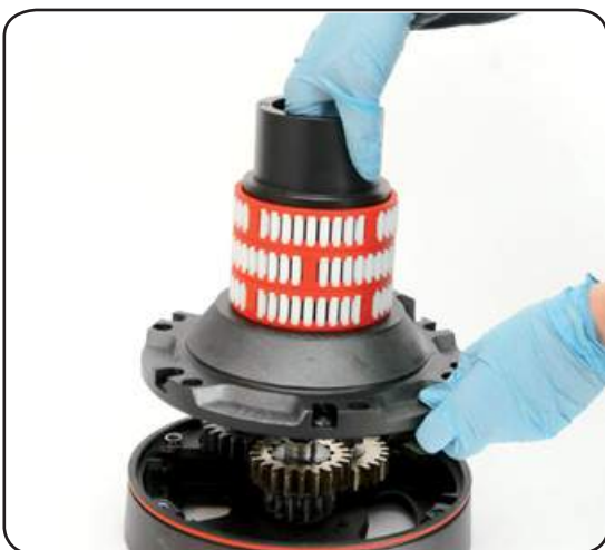
10. Remove the drum support n°16 Important: washer n°7 may remain inside the drum support!
