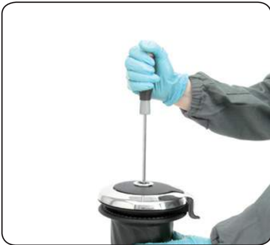
1. Unscrew the central screw ( \approx 2\text{Nm}/18\text{ in-lb} )
