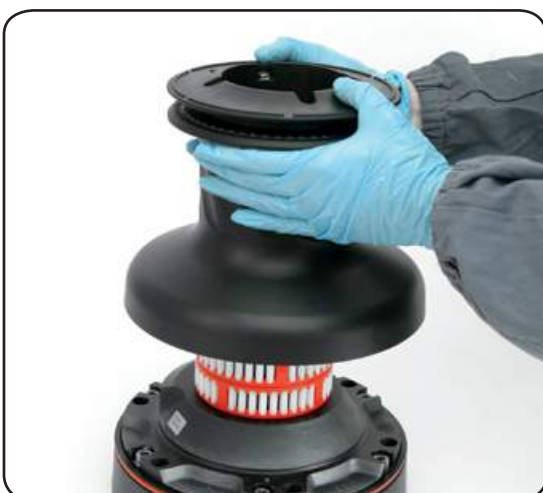
5. Lift off the drum n°24
