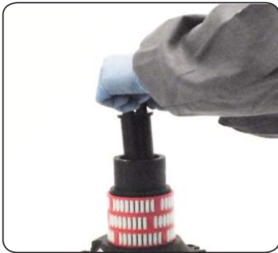
7. Slide out the assy clutch n°37
