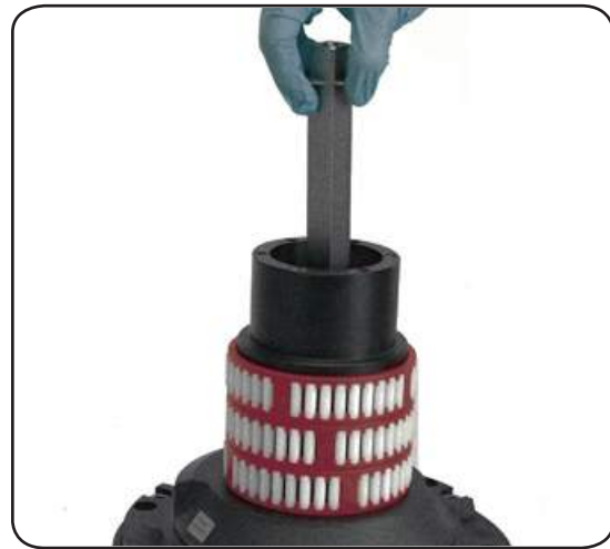
8. Slide out the central shaft n°19
