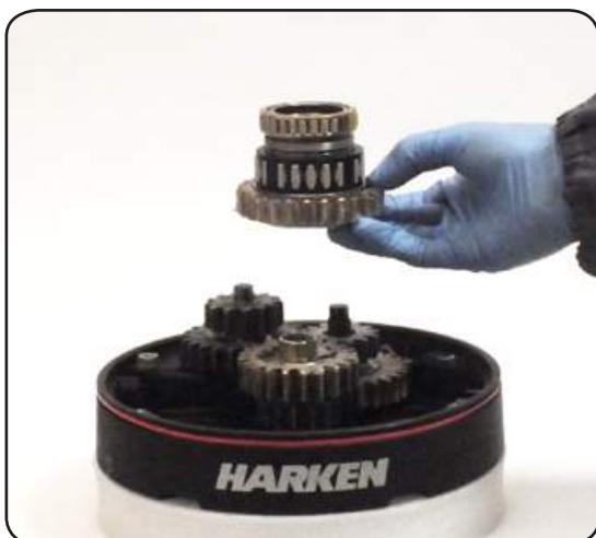
11. Remove the gear n°31, pawls carrier n°33, the bearings n°34 and 36 and the pin n°35 Important: washer n°7 may remain inside the drum support!
