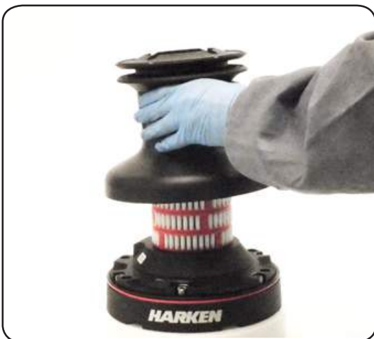
5. Lift off the drum n°24
