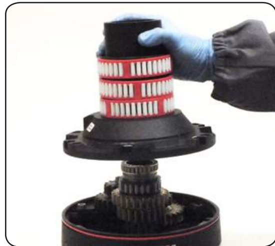
10. Slide out the drum support n°16
