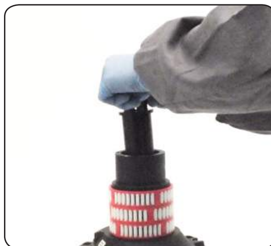
7. Slide out the assy clutch n°37
