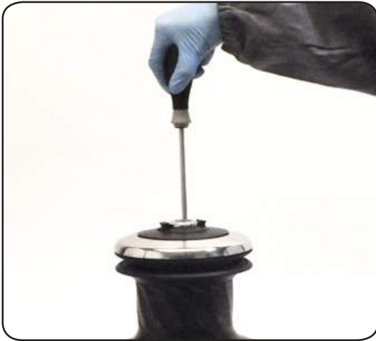
1. Unscrew the central screw (🔧2Nm/18 in-lb)
