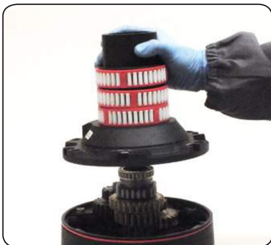
10. Remove the drum support n°16
