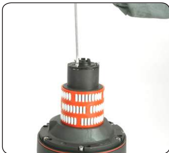
6. Completely unscrew the three screws n° 28
