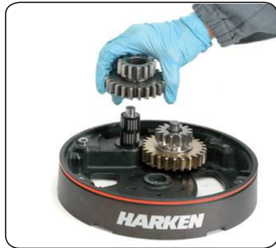
13. Remove the idler and pinion n°14
