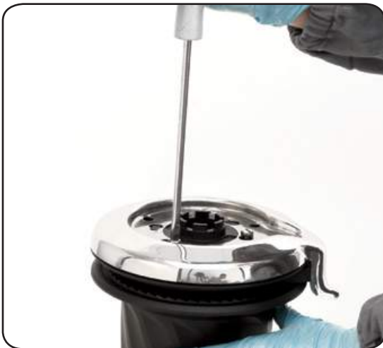
3. Unscrew the three screws n°28 (⚙️4Nm/35 in-lb)
