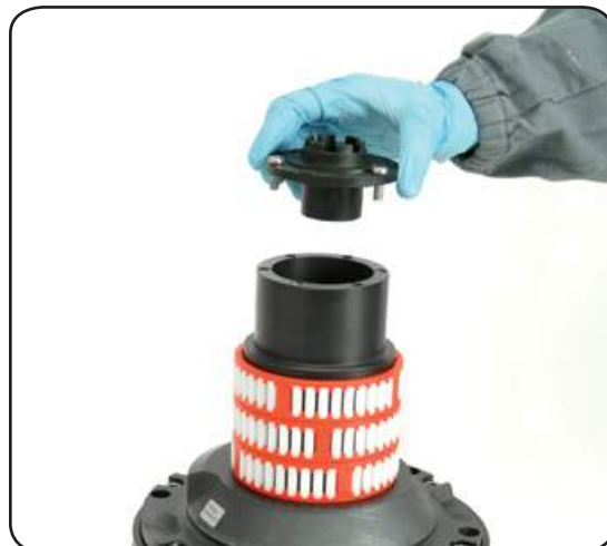
7. Remove the stripper arm housing n°21
