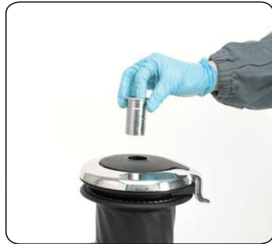
2. Slide off the assy socket n°30 and the cover 29
