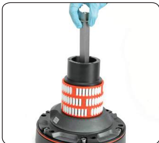
8. Slide out the central shaft n°19
