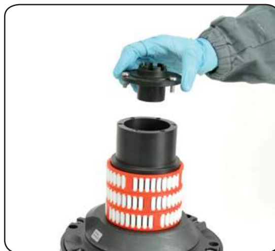
7. Remove the stripper arm housing n°21
