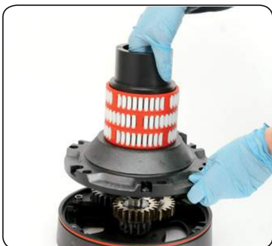
10. Remove the drum support n°16
