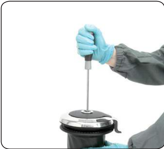
1. Unscrew the central screw (⚙️2Nm/18 in-lb)
