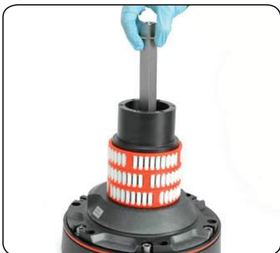
8. Slide out the central shaft n°19
