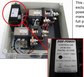
Use a small Flathead or Phillips head screwdriver to adjust the timer delay located in the top right-hand corner of the Series/Parallel Switch Box. To decrease the Soft Start timer delay to the minimum of 1/2 second, turn the adjustment screw counter-clockwise until it stops. To increase Soft Start timer delay, turn the adjustment screw clockwise.
