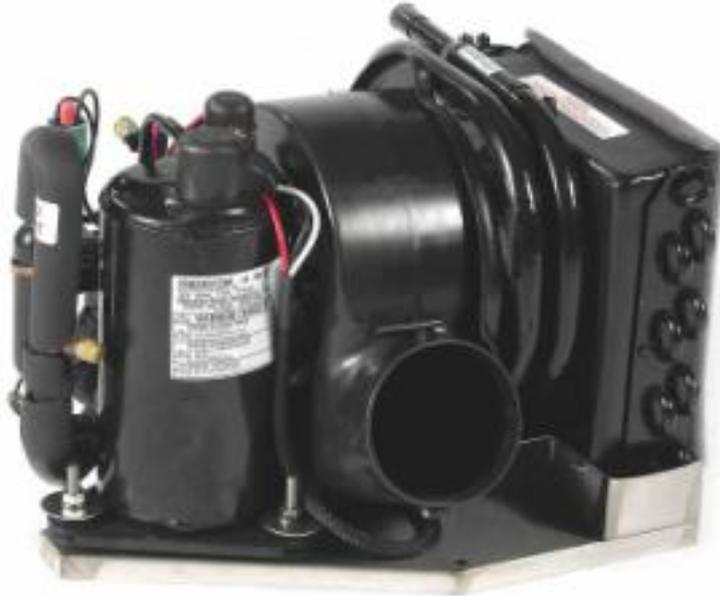
Smallest footprint on the market and weighs in at 31.5 lbs. for the unit, and 4.7 lbs for the electrical box! This unit has a rotatable blower and tapers down to a "V" shape for those odd angle discharge installations. We use 4" ducting and recommend a minimum of 2, 4" round supply grills with this installation.
