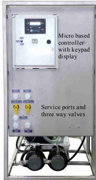
Micro based controller with keypad display
