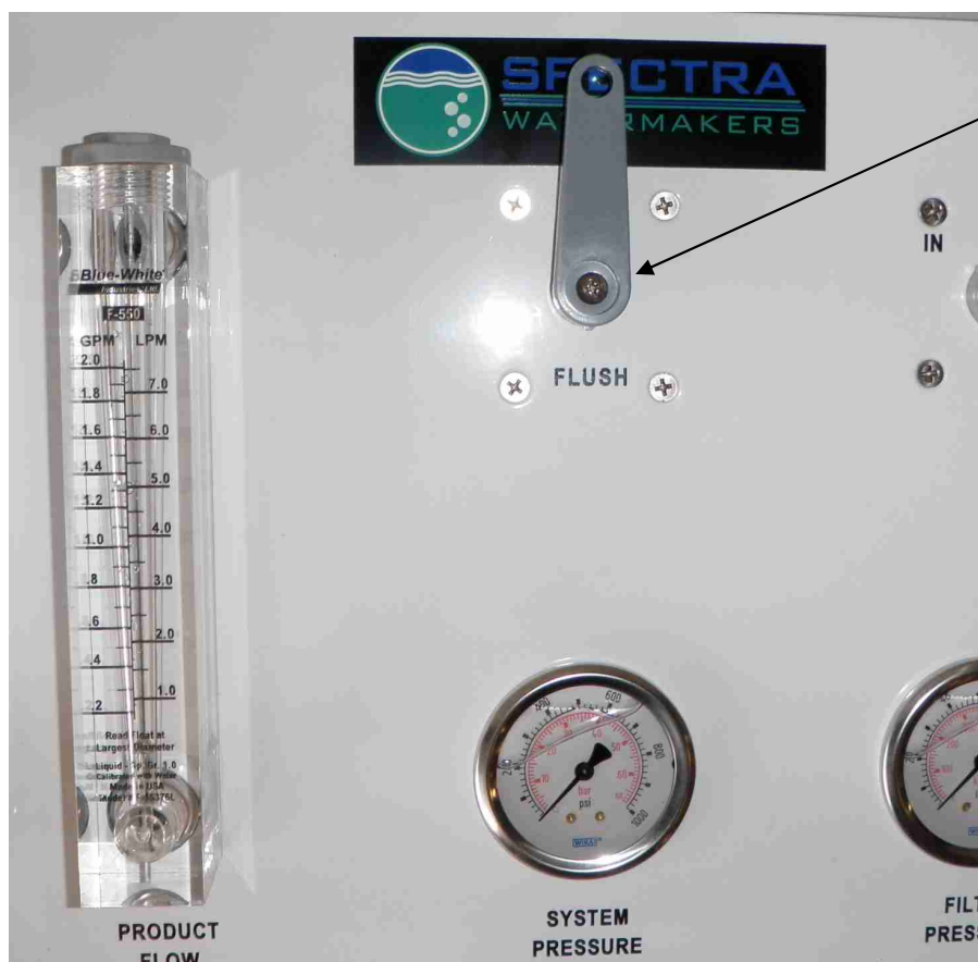
Flush Valve in 'Fresh Water Flush' position
